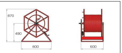
Designed for sub-sea main line hose connection between the pump and the first tensioner, the reel above is suitable for off-shore use and can accommodate up to 300 meters of Hi-Force XHC hydraulic hose. The reel comes complete with quick connect couplings, integrated brake and a spring loaded locking bolt.
