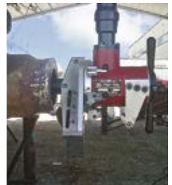
SDB end prepping pressure vessel
