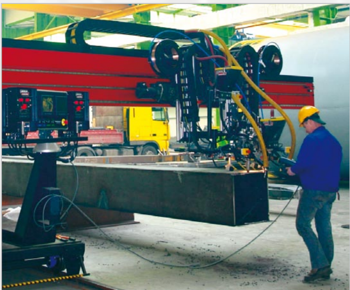
Standard Column & Boom with ESAB Aristo 1000 AC/DC
