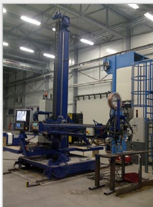
Standard Column & Boom with ESAB Aristo 1000 AC/DC
