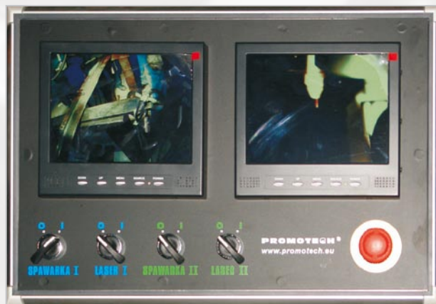
Optional equipment includes: camera system for GMAW/ SAW, automatic correction of welding gun position or remote control.
