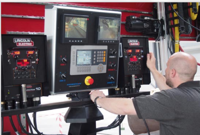
Half Gantry Beam and Tank Welding System C&B type WA with LINCOLN ELECTRIC PW AC/DC 1000 SD
