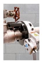
The Wachs Small Diameter Split Frame (SDSF) tooling works in all machine models from 1/2in (DN 15) up to 6in (DN 150). The cut and bevel form tools can machine all common pipe materials and most pipe schedules up to .437in (11.11mm) wall. The socket weld tooling covers the same size pipe sizes and sockets up to 6,000 lbs (2721kg).
