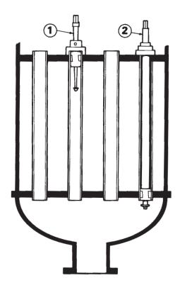
The diagram above illustrates: (1) an "SB'parallel rolling type expander to locate and seal the tube in the upper tube plate and (2) the long-body Sugar Refinery expander operated from the upper tube sheet area.
