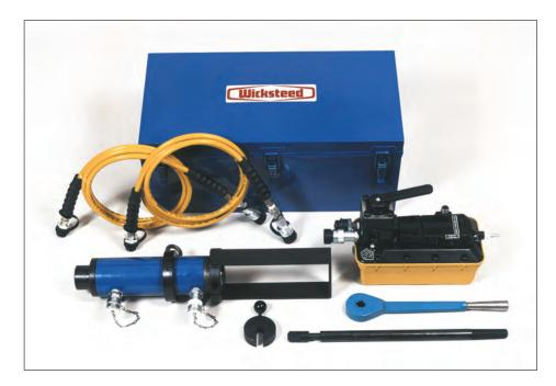
The 20 Tonne Portable Tube Stub Removal Kit offers a more powerful and efficient method of removing tube stubs up to 1" (25.4mm) in dia, by means of a double acting hydraulic cylinder giving powered movement in both directions.
